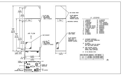
As standard, all ML Series supplies provide output VOLTAGE AND CURRENT PROGRAM/MONITOR (0-+10V = 0-fs), HIGH VOLTAGE ENABLE (0-1.5V off, 2.5 -15V on), HIGH VOLTAGE STATUS (high = HV on, low = HV off), SAFETY INTER-LOCK (open = off, closed = on), CUR-RENT TRIP/LIMIT select, +10 VOLT REF-ERENCE source, V/I MODE STATUS (high = voltage mode, low = current mode), LOCAL CONTROL, COMMON and CHASSIS GROUND.
