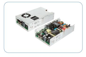
The PBR500 series of AC-DC switching power supplies, in a package of just 4 x 7 x 1.7 inches, deliver 450-500 watts of continuous power with forced air cooling or 350-400 watts with convection cooling. The units are constructed on a U-Channel for mechanical support and heat sinking. A cover and fan assembly can be added during manufacturing. They are designed for both ITE/Industrial and medical applications including those needing BF rated insulation with an operation altitude up to 5000 meters.
