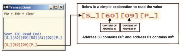
It is then required to convert the hexadecimal data into decimal and insert a decimal place in the appropriate place to get the actual voltage measured. Follow the conversion steps below:
