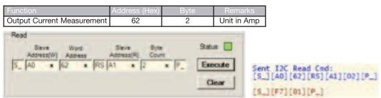
Converting 01F7<sup>h</sup> into decimal gets 0503<sup>d</sup>, and dividing by 100 as previous, and the resulting current measurement is 5.03A. Below is the actual measurement captured on a meter.
