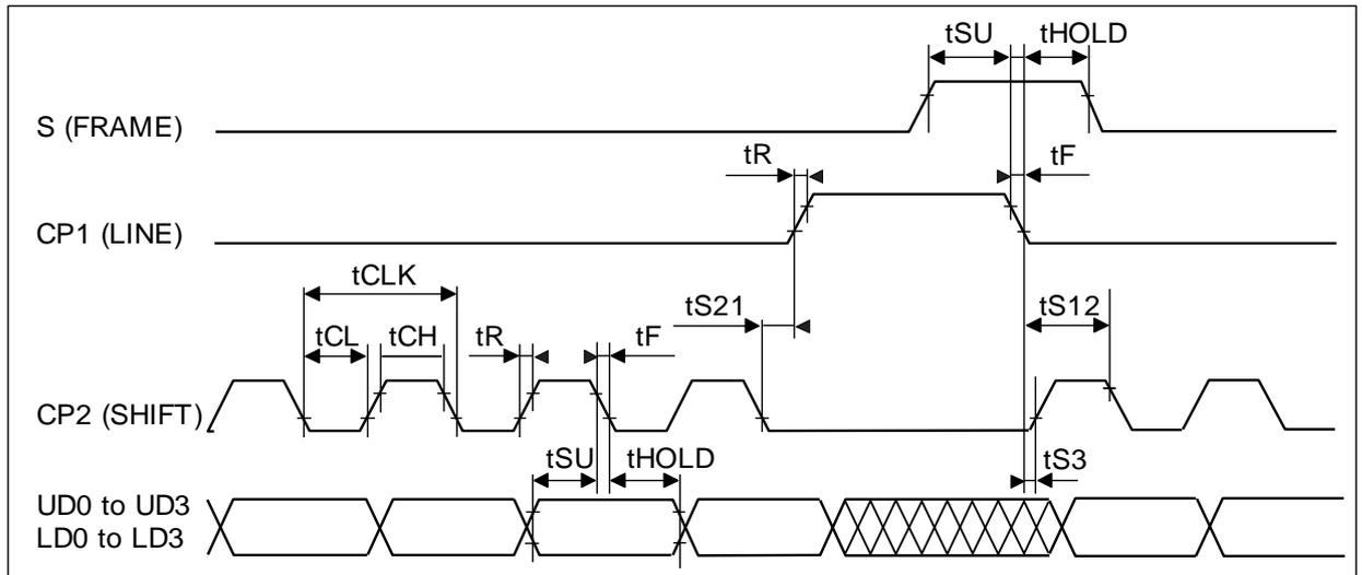
**Figure 5. Setup and hold timing diagram**
