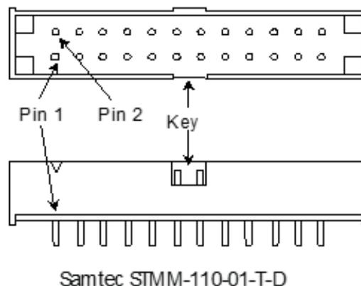
**Figure 1. AG1 Data and power connector**
