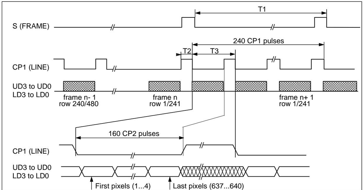
**Figure 4. Video input timing diagram**
