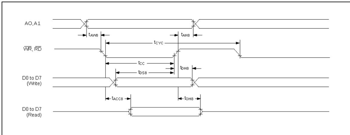
**Figure 3. 8080 video input timing diagram**
