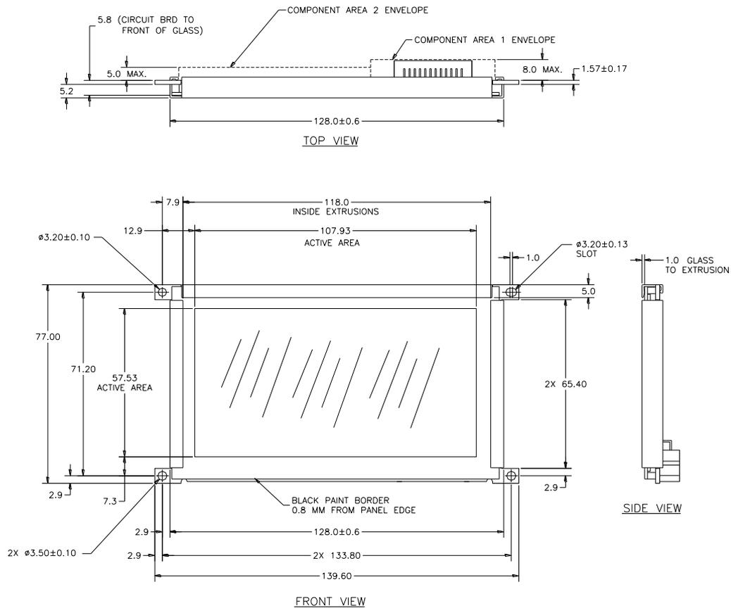
Dimensions are in millimeters.
