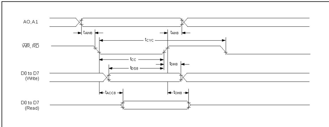
**Figure 4. 6800 Video input timing diagram**
