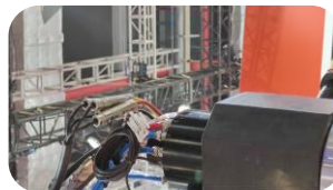
motor encoder and circular power connector
