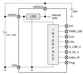
Figure 16: Connections for 5V / 3.3V supply voltages
