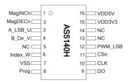
Figure 2: Pin configuration SSOP16
