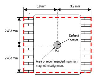
Figure 18: Defined IC center and magnet displacement radius
