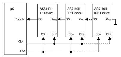
Figure 5: Daisy Chain hardware configuration
