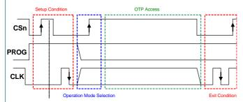
Figure 13:OTP access timing diagram
