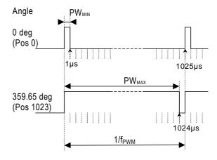
Figure 9: PWM output signal
