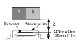
Figure 19: Vertical placement of the magnet
