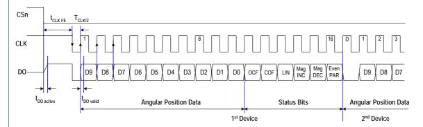
Figure 6: Daisy Chain mode data transfer
