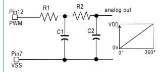
Figure 10: Simple passive 2nd order lowpass filter
