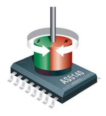
Figure 1: Typical arrangement of AS5140H and magnet
