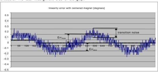
Figure 22: Example of linearity error over 360°
