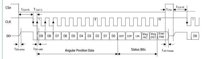
Figure 4: Synchronous serial interface with absolute angular position data
