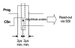
Figure 14: Enabling the alignment mode
