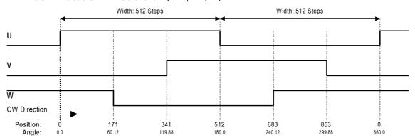
Figure 11: U, V and V-signals for BLDC motor commutation (Div1=0, Div0=0)
