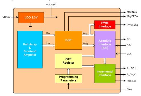
Figure 3: AS5140H block diagram
