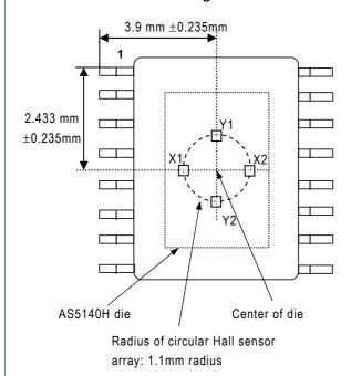
Figure 20: Arrangement of Hall sensor array on chip (principle)
