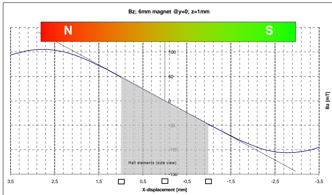
Figure 23: B_z field distribution along the x-axis of a 6mmØ diametric magnetized magnet
