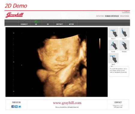
The 2D demo screen is an example application that illustrates how easy it is to position and size an image for viewing using the MTCW. Use a single finger (or two fingers) on the touchpad to pan the image in the X or Y direction. Use two fingers in a pinching or un-pinching motion to control the zoom level. Spin two fingers about each other to rotate the image.
