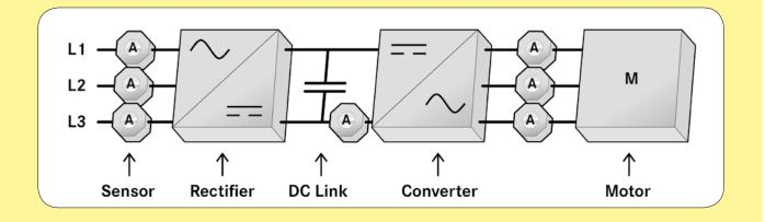
Frequency converter for Generator-Grid connection
