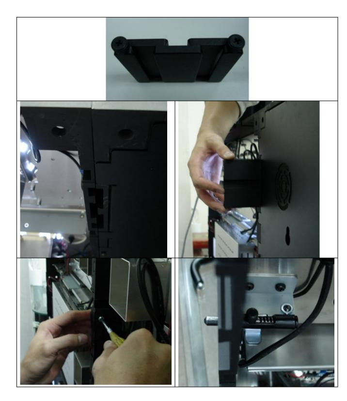
Similarly, the grub screws in the base can be used to adjust the height of the modules, but make sure not to exceed the available length on the grub screw. These are intended for fine adjustments only.
