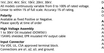
180-250VAC three phase 50A max, or 340-460VAC three phase 25A max, contact factory for 480VAC. Unit includes field conversion kit for 208 to 400VAC or 400 to 208VAC.
