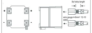
9.5mm fast-on tags Amp 151667-2 max 32A per terminal, depending on wire crimp tool Vogt 3975C
