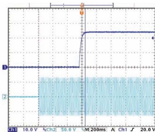
Figure 2 - V1 Start up examples from AC turn on
