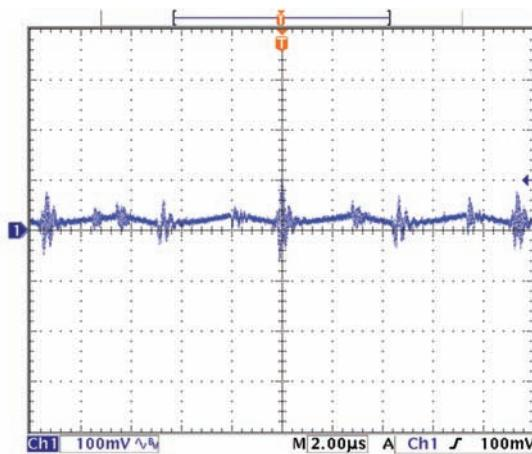
Figure 4 - V1 HPU1K5PS24 (Full load) 160mV pk-pk
