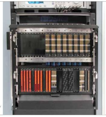
Avionics Circuit Card Tester with 9050 VXI
