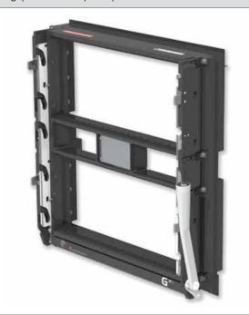
The G40x Pull-Thru receiver is a two tier, 48 module system that enables pull through removal of 40 VPC modules, InterConnect Adapters, and test instrumentation in one piece. It offers eight standard 90 Series module slots, plus space for two iCon modules, as needed. The G40x Pull-Thru is slide mounted, to enable easy access to the discrete-wiring modules.
