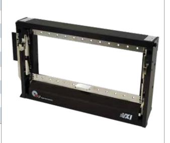
The 25 module VXI receiver allows you to use 12 pre-wired InterConnect adapters. It also hinges down for direct access to the instruments. It is equipped with a locking handle to ensure your contacts are engaged. A standard integrated microswitch shuts off power when the ITA disengages from the receiver.
