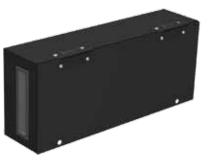
The 20 module enclosure is made of aluminum, painted black, and secured to the ITA by eight socket head cap screws (included). It has a depth of 4".
