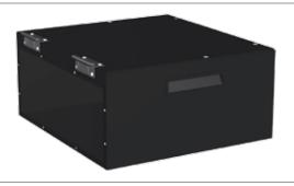
Made of aluminum, the enclosure body is painted black and features a hinged cover plate with 1/4 turn hardware that provides easy access to the ITA wiring. The enclosure is secured to the ITA by 12 #4 socket head cap screws.
