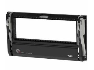
The 25 module receiver is designed to fit into a standard 19" rack. It is equipped with a locking handle to ensure your contacts are engaged. A standard integrated microswitch shuts off power when the ITA disengages from the receiver.
