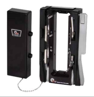
The G2 receiver is equipped with a locking handle and nickel plated steel slides that engage up to 400 contact points. It allows a high amount of I/O within a compact and rugged device. A protective cover is included with the receiver.
