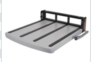
The 20" G12 receiver provides a large platform for use with large fixtures. When used in conjunction with VPC slide mounts and support legs, the receiver can support 350 lbs. The G12 handle can be rotated in 90 degree increments. Also available in a 15" platform, Part # 310 104 325.
