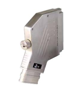
The i2 MX ITA accepts two module inserts, which allows a variety of signal, power, coax, thermocouple, and fiber optic connections. The cable exit is one inch in diameter. Pre-configured receivers are also available. For more information, please refer to the previous exploded-view diagram on page 41.
