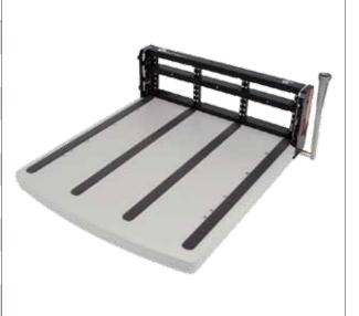
The G12x receiver 20" platform will support 180 lbs when used in a slide mount configuration. The receiver is equipped with VPC's Quadratrack™ engagement system which provides four points of pull down for a reliable connection every time beyond 20,000 cycles. It can accept both the G12 and G12x ITAs. The G12x handle can be rotated in 90° increments. Also available in a 15" platform, Part # 310 104 386.
