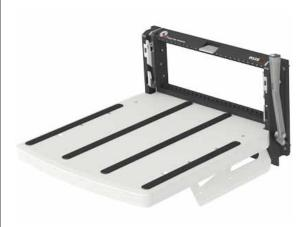
Runners along the platform provide a smooth-sliding action, ideal when using fixtures up to 180 lbs. When used in conjunction with VPC slide mounts and leg kit, the receiver can support 350 lbs. The 9025TR can be adapted to accommodate vacuum or mechanical fixturing. The 9025TR uses all standard 90 Series modules and contacts, includes a microswitch and is available with optional leg and keyboard tray kits. A slide kit is required for use.
