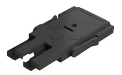
Blank inserts are for unused SIM insert slots. One blank insert fills a SIM single insert slot and fits in either receiver or ITA 90 Series modules or the i2 MX. Ten blank inserts are included per part number.
