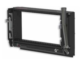
The G20 Pull-Thru receiver offers direct connection to instrument modules, enabling pull through removal of connector modules and instrumentation from the chassis backplane.
