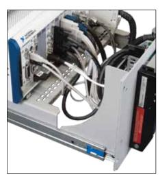
Figure 2 Cable Tie Down Bar on Instrument Bracket
