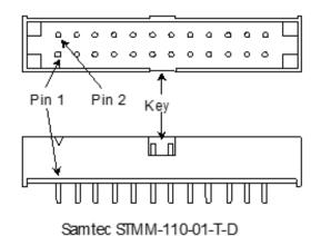
Figure 1. AG1 Data and power connector
