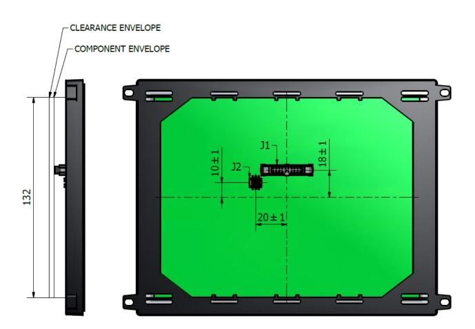
Dimensions in are millimeters; inches in brackets. Tolerances, unless otherwise stated,  $\pm$  0.2 mm. Connector is shown from the back side.
