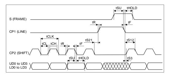
Figure 5. Setup and hold timing diagram
