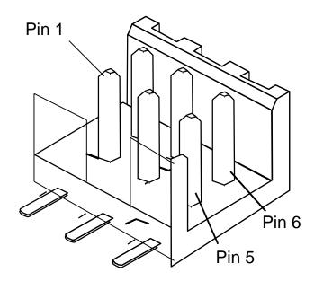
Figure 3. AG1 ET Dimming connector: FCI 98424-G52-06A
