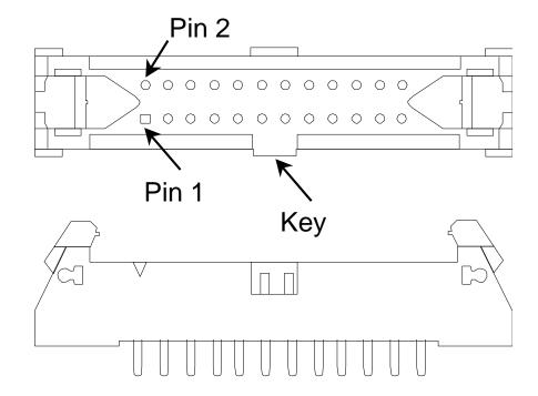
Figure 2. AG1 ET Data and power connector: Samtec EHT-110-01-S-D
