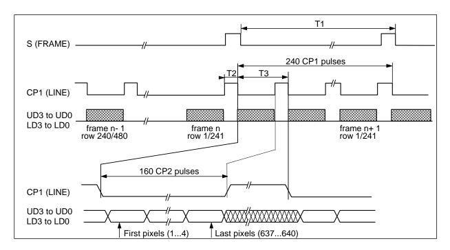
Figure 4. Video input timing diagram
