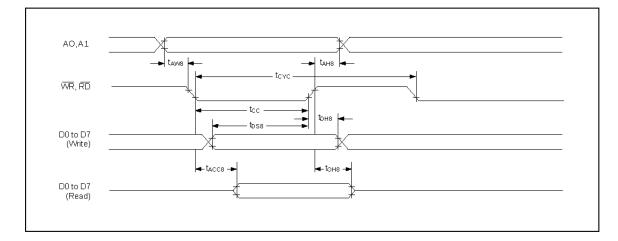
Figure 3. 8080 video input timing diagram
