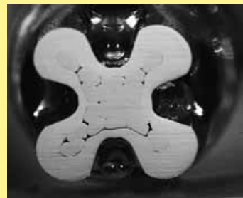
Crimp-cross section HARTING crimp profile
