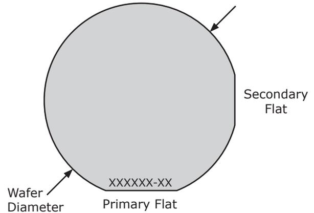
Figure 1. Diameter and Primary and Secondary Flat Dimension
